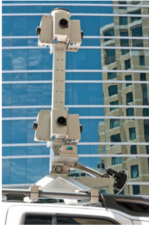
Figure 3-1: The Earthmine Mars Collection System collects high resolution stereo panoramic imagery. Copyright Earthmine Australia 2015.
