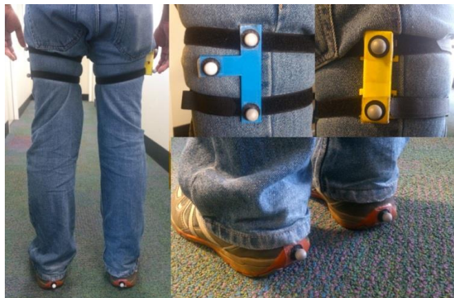
Figure 5.8 – Marker and IMU placement on legs
