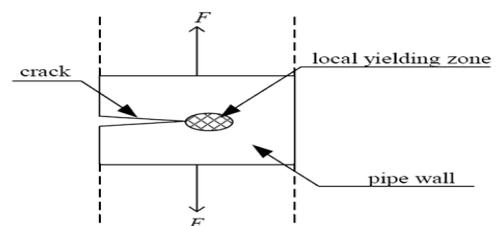
Figure 8. Local Yielding Zone at Crack Point
