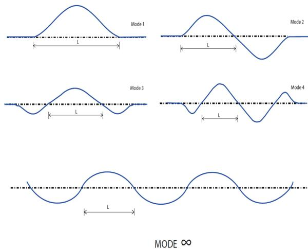
**Figure 3.** Lateral Buckling Mode Shapes
