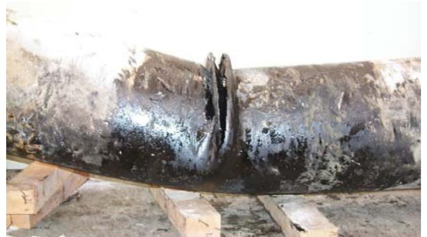
Figure 7. Example for Rupture Failure Mode under Bending (Palmer)
