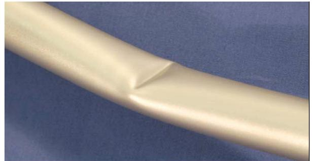
Figure 6. Example for Ovalisation Failure Mode under Bending (Kyriakides et al)
