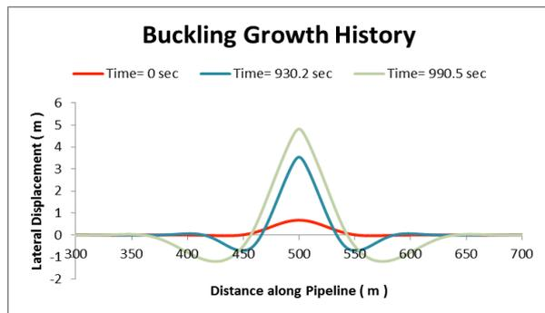
Figure 5. Lateral Deformation Response
