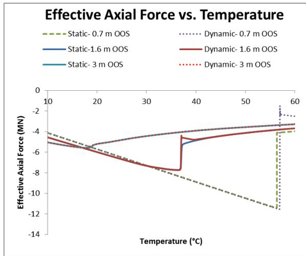
Figure 23. Effective Axial Force versus Temperature
