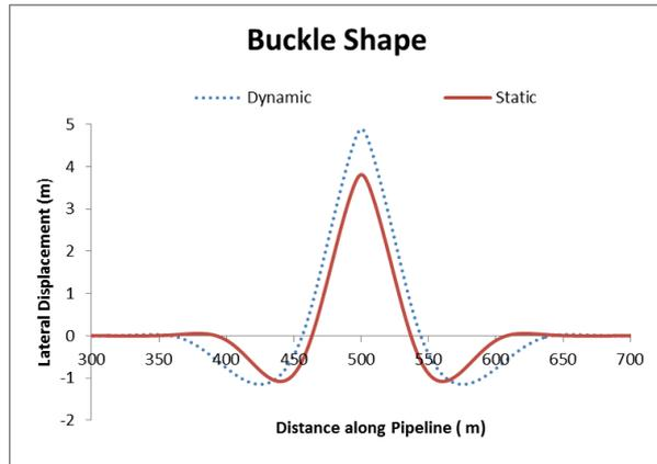
Figure 17. Buckle Shape for Static & Dynamic Cases @ Maximum Operating Temperature- Heavy Pipe
