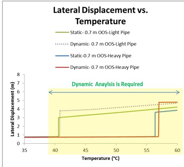
Figure 16. Lateral Displacement versus Temperature
