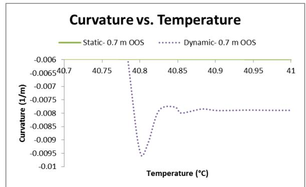
Figure 19. Curvature versus Temperature for Dynamic Case using 0.7 m OOS for Heavy Pipe during Snap-Through
