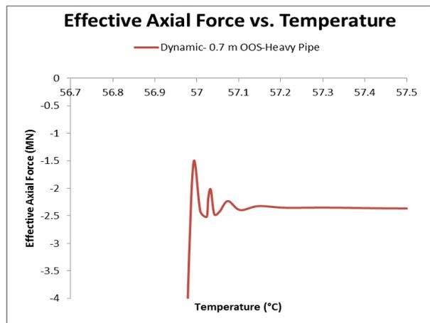
**Figure 15. Effective Axial Force versus Temperature for Dynamic Case using 0.7 m OOS for Heavy Pipe during Snap-Through**
