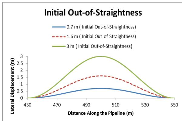
**Figure 12.** Initial Horizontal Out-of-Straightness
