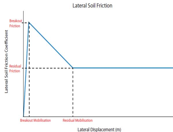
Figure 10. Example for Tri-Linear Response-Lateral Friction Factor
