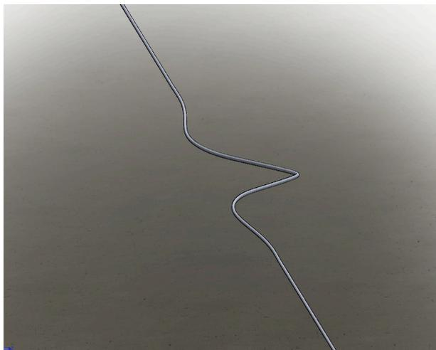
Figure 1. Buckled Pipeline on a Flat Seabed
