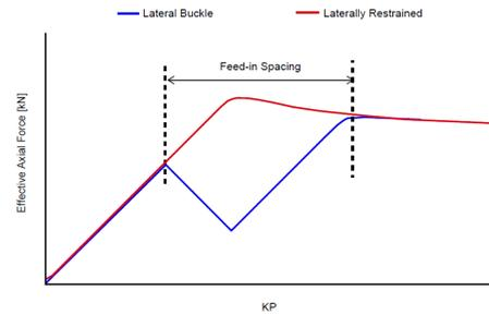
**Figure 13.** Illustration of Virtual Anchor Spacing
