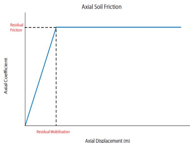
Figure 11. Example for Bi-Linear Response-Lateral Friction Factor
