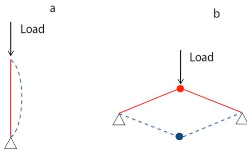
**Figure 2.** Buckling Schematics: (a) Symmetric Bifurcation (b) Snap-Through Buckling
