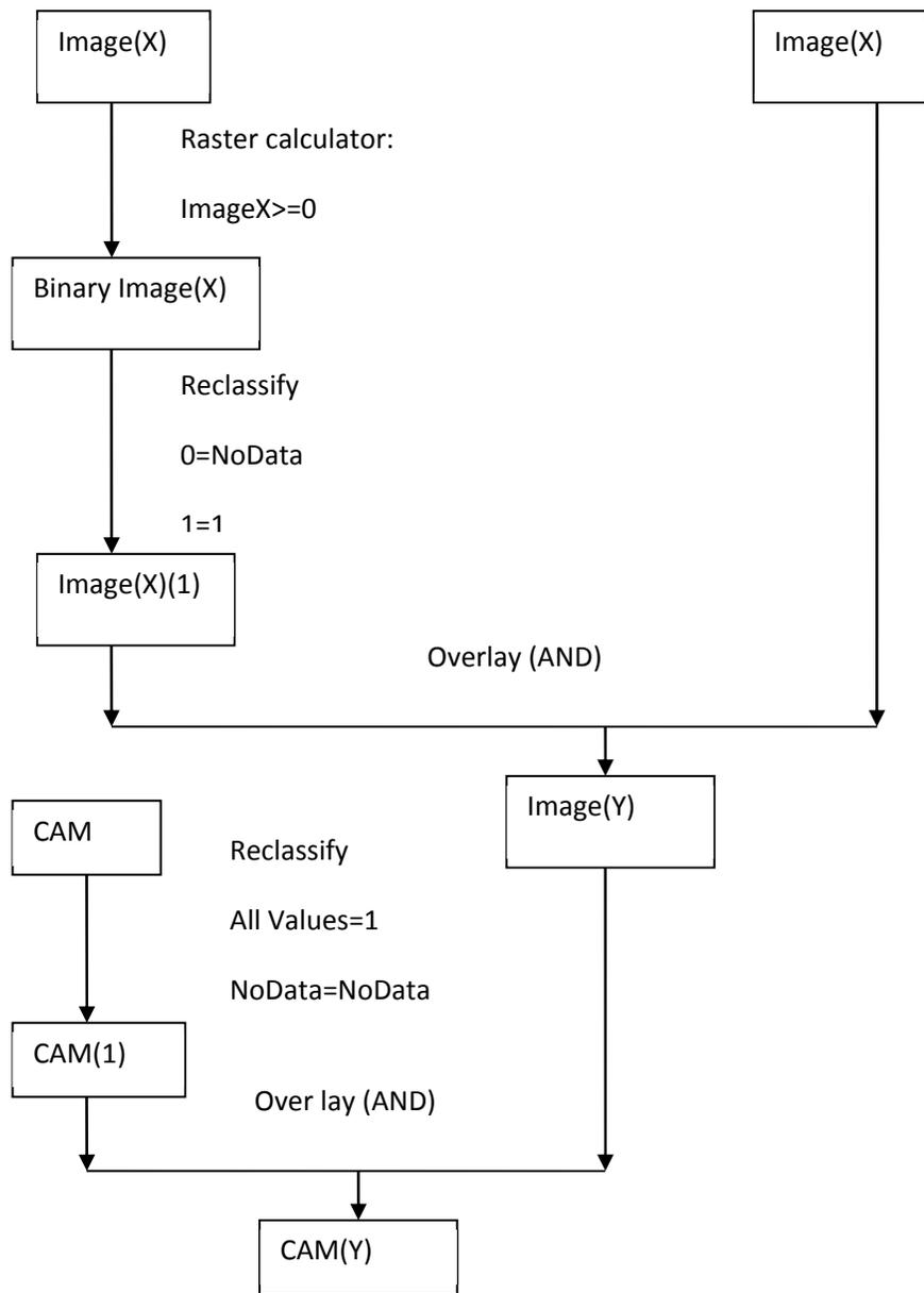
Figure 4: Processing structure chart for the GIMMS NDVI images.
