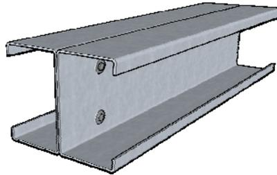
Figure 1: Lipped Back-to-back Built-up I Sections
