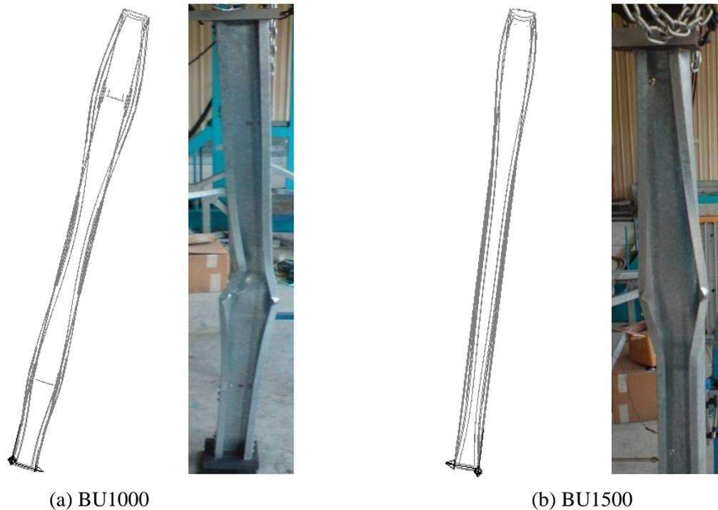
Figure 8: Deformed Mesh in FEA and buckling in Testing
