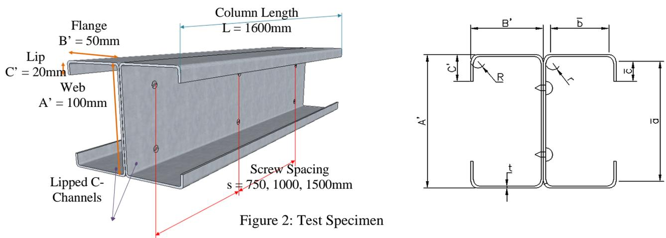
Figure 2: Test Specimen
