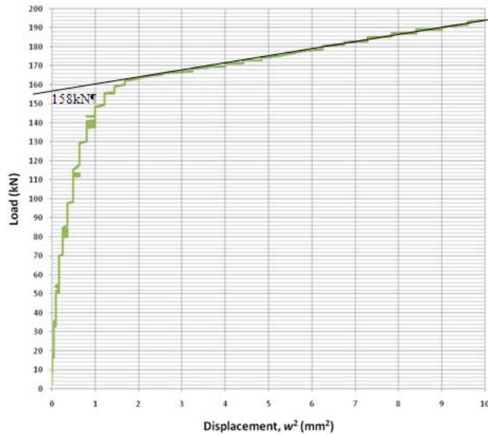
Figure 4: Load vs the square of local buckling deformation for BU1000-1
