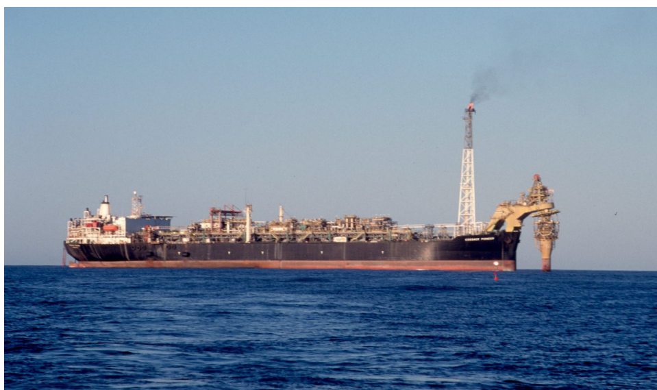
Fig. 1. (Color online) Photo of the Cossack Pioneer FPSO (bow attached to riser on the right side of the picture).
