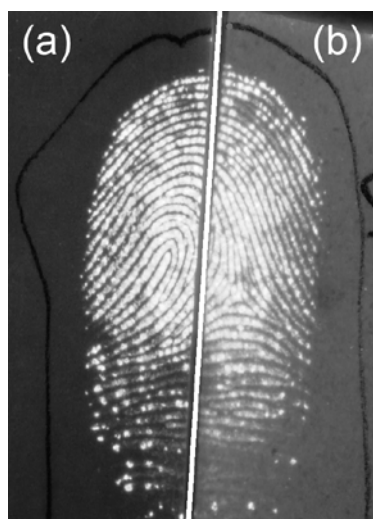
Fig. 3 Fingerprint treated with (a) 1 mL of stock solution (1 g DMAB in 22 mL ethyl acetate and 0.5 mL acetic acid) in 9 mL HFE-7100 and (b) 0.6 g DMAB in 49.5 mL ethyl acetate and 0.5 mL acetic acid. Photograph taken with a Nikon D300 camera in luminescence mode; focal length: 60 mm, shutter speed: 1 second and aperture: f/11.
