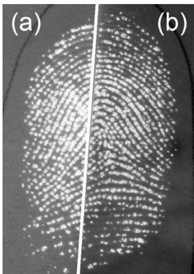
Fig. 4 Fingerprint treated with DMAB working solution, (a) heated in an oven and (b) an Elna laundry press. Photograph taken with a Nikon D300 camera in luminescence mode; focal length: 60 mm, shutter speed: 1 second and aperture: f/11.
