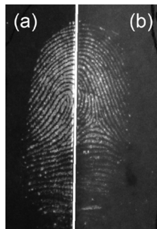
Fig. 10 One month old fingerprint treated with (a) IND/ZnCl 2 and (b) DMAB working solution. Photograph taken with a Nikon D300 camera in luminescence mode; focal length: 60 mm, shutter speed: 1 second and aperture: f/11.
