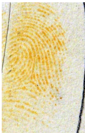
Fig. 2 Fingerprint treated with DMAB working solution. Photograph taken with a Nikon D300 camera in absorbance mode; focal length: 60 mm, shutter speed: 1/20 second and aperture: f/11.
