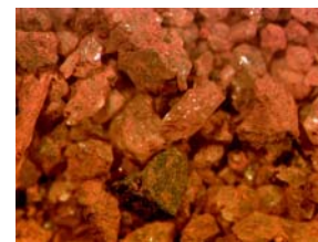
Fig. 2 Optical microscopy image of the bauxite residue sand magnified 30 times
