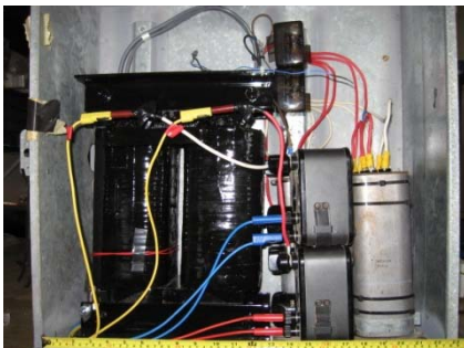
Figure 6 bench testing of reactor quality factor and temperature rise
