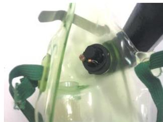
Fig. 6. ITAB mounted on an oxygen mask.
