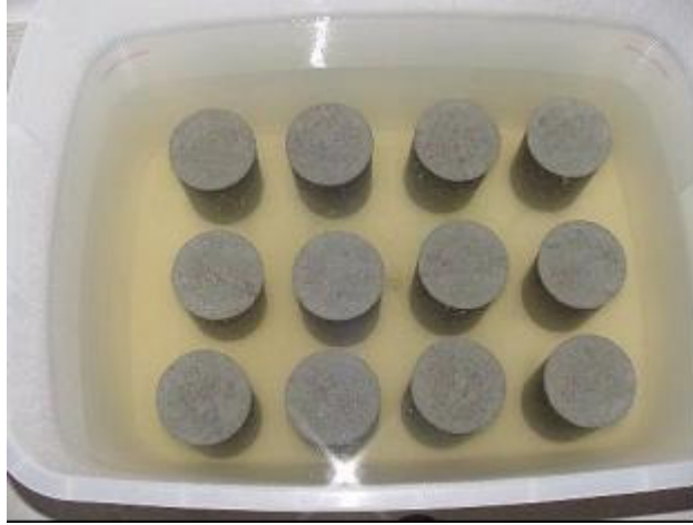
Figure 3.18 Specimens Soaked in Sodium Sulfate Solution
