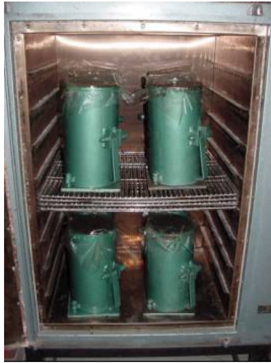
Figure 3.9 Dry (oven) Curing
