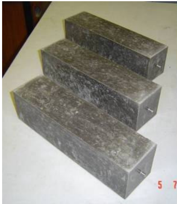
Figure 3.15 Specimens for Drying Shrinkage Test
