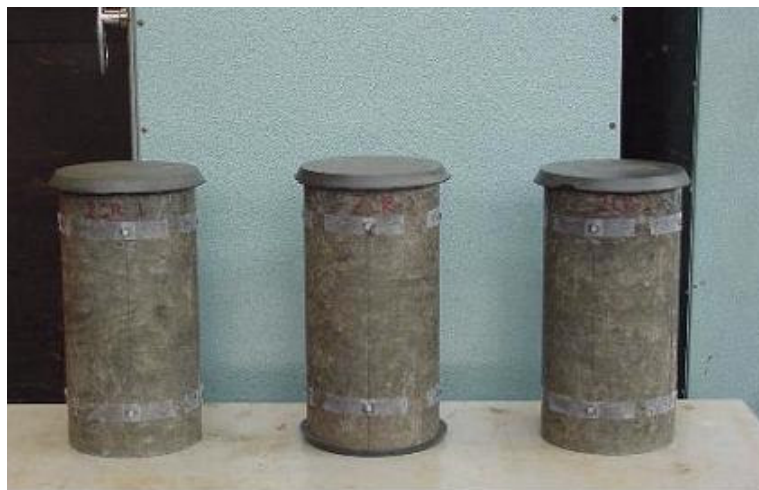
Figure 3.11 Creep Test Specimens
