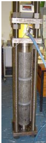
Figure 3.13 Creep Test Set-up
