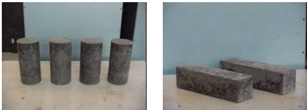
Figure 3.17 Specimens for Sulfate Resistance Test
