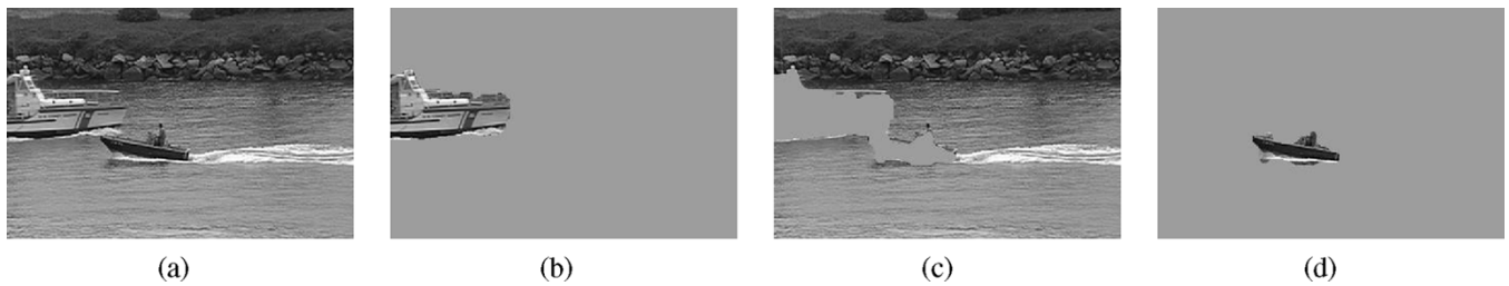
Fig. 15. (a) One frame of the “coastguard” sequence. (b)–(d) Video segmentation results.
