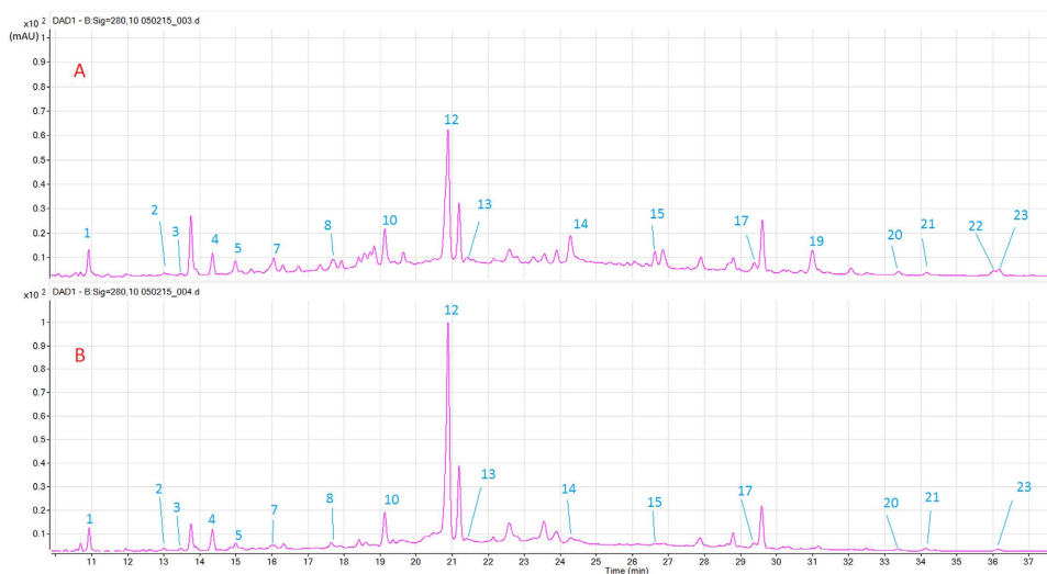
Figure 1. Representative chromatograms of sorghum whole grain phenolic compounds (A) Free phenolic compounds from genotype CHH2 grown at OT. (B) Free phenolic compounds from CHH2 grown at HT.
