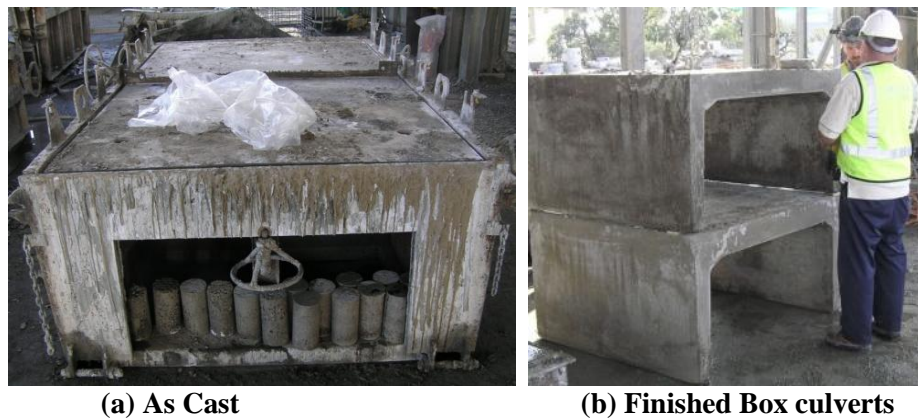
Fig. 3. Manufacture of Test Culverts and Cylinders
