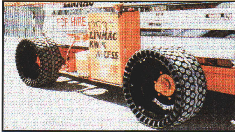
Figure 3.11 Tyres fitted to scissorlift platform.
