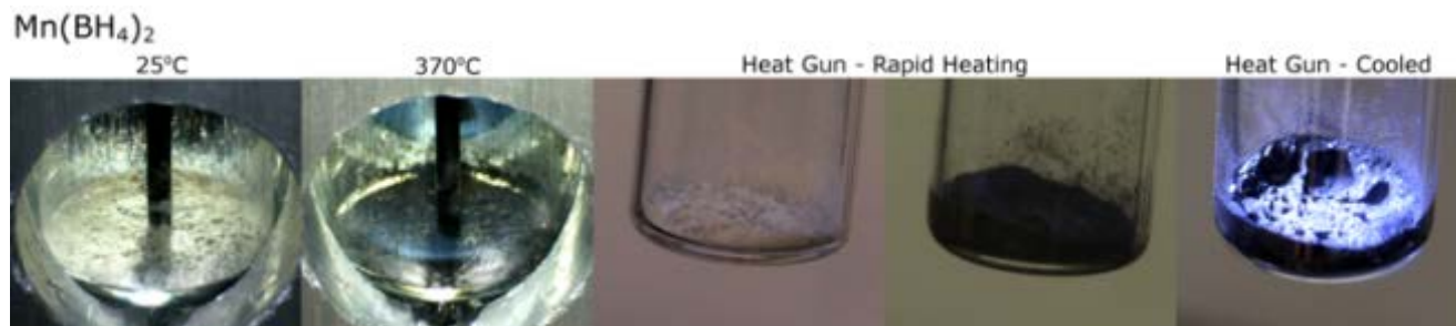
Figure 9: Photographic sequence during thermolysis of \text{Mn}(\text{BH}_4)_2 at 10\text{ }^\circ\text{C}/\text{minute} under argon and evolved gases maintained at 1 bar. Photographs are also shown of a sample heated rapidly at an uncontrolled heat rate using a hot air heat gun.
