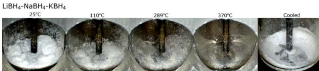
Figure 23: Photographic sequence during thermolysis of 0.45\text{LiBH}_4\text{-}0.1\text{NaBH}_4\text{-}0.45\text{KBH}_4 at 10\text{ }^\circ\text{C}/\text{minute} under argon and evolved gases maintained at 1 bar.
