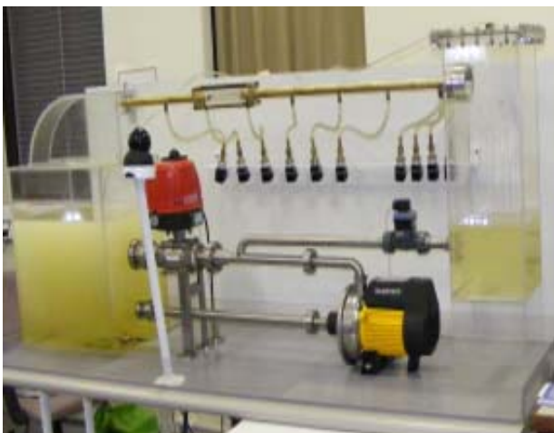
Figure 2. Remote laboratory equipment for the study of the flow through a pipe
