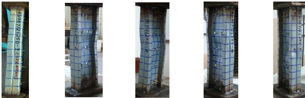
BU75T12L250-1 BU75T12L250-2 BU75T12L250-3 BU75T12L250-4 BU75T12L250-5 Fig. 3 Failure Modes of Tested Specimens
