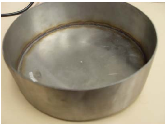
Figure 2. Metal Container used for cracking test
