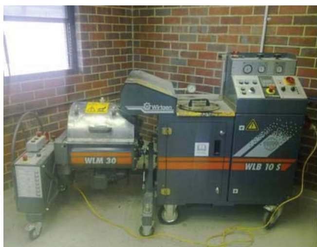
Figure 4. Wirtgen WLB 10S (right side), with a mixer WLM 30 (left side).
