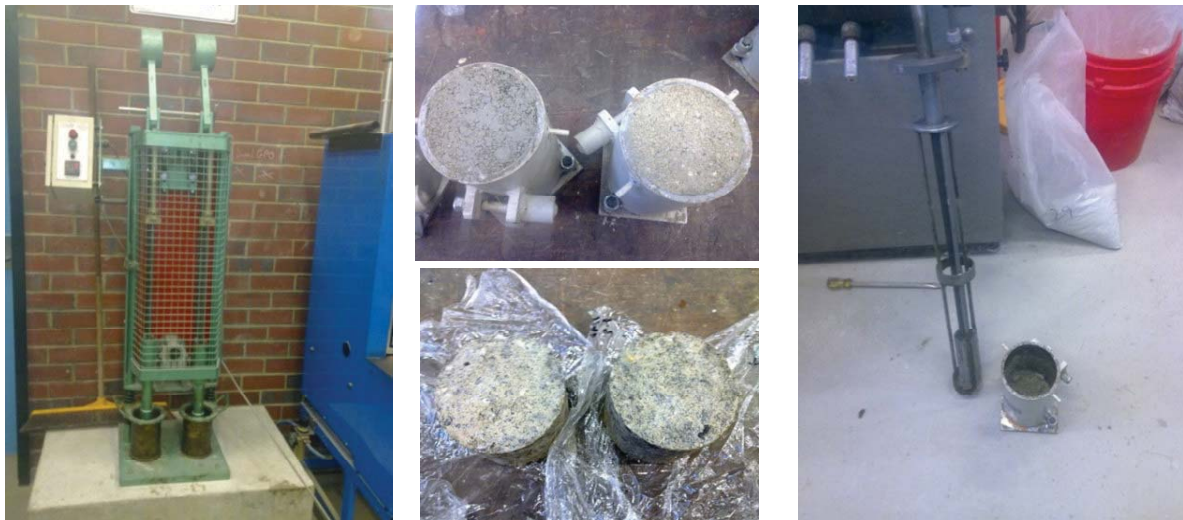
Figure 6. Automatic marshall compactor and modified compaction tools.
