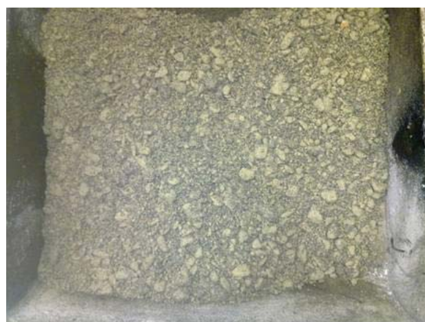
Figure 5. A mixing example of 5% foamed bitumen with 75% CRB and 25% CLS.
