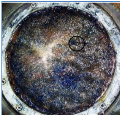
Fig. 3 Deformation of GCLs surface
