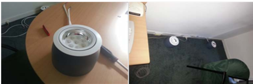
Figure 7.4 The lighting fixtures which were designed to direct the RGB LED down-light upwards onto the walls of the hotel room.
