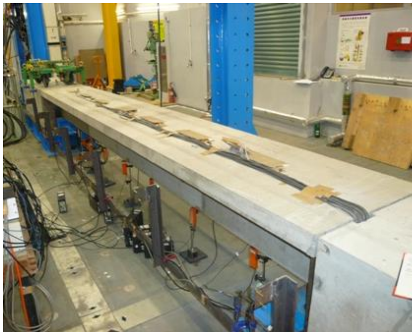
(b) Optical triggers and accelerometers
