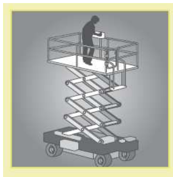
Figure A.12: Scissor-lift elevating Work platform
