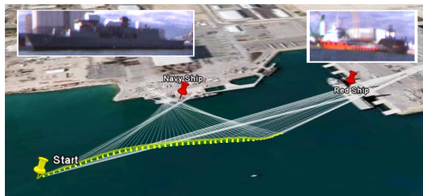
Figure 6. Port Facility. Trajectory of the platform (yellow path) and bearings (white lines) towards the stationary target objects. The positions of the stationary targets have been registered manually.
