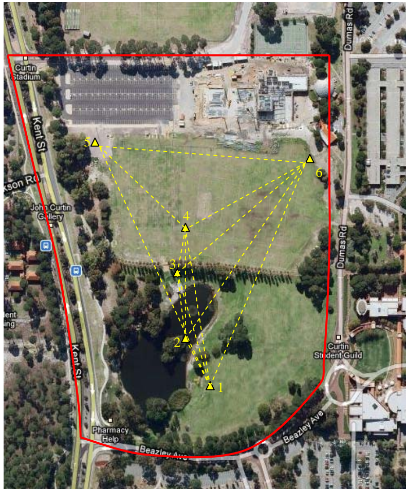
Figure 3: The Curtin study area with the control peg network. The distances between pegs are listed in Table 1 ( http://maps.google.com/maps ).
