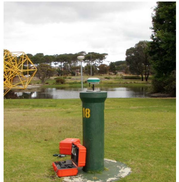
Figure 4: Left: The Curtin GNSS Baseline Network Pillar locations within the study area. Right: Base receiver setup on Pillar 18.
