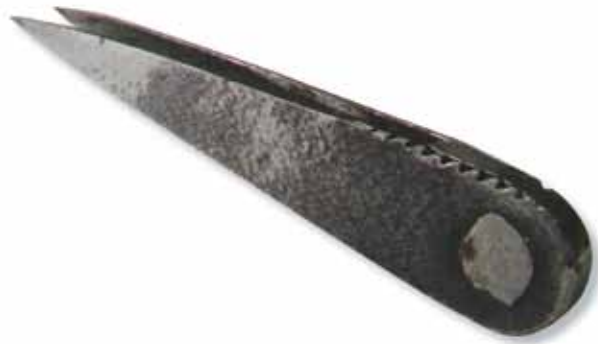
Figure 22 In the 1970s a recycled hacksaw blade was turned cleverly into these foreigner tweezers. Photograph by Gina Pickering.
