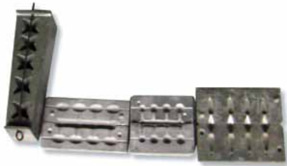
Figure 25 These patterns which are thought to be for sinker moulds (c.1950) have been identified as foreigners. It is not always possible to identify a foreigner, especially among the hundreds of patterns which were some of the easiest foreigners to hide. As they were often used many times, they were likely to be left on-site with the maker being spared the ordeal of smuggling them out.
