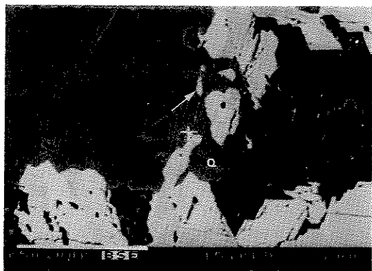
Fig. 11. BSE image showing the intergrowth between S2 cement (white) displaying characteristic rhombs and quartz overgrowths (medium grey). Locally the siderite is completely engulfed by the quartz cement (arrow), indicating that some siderite cementation preceded quartz (Q) cementation. Sample F1-9433, Fly Lake 1, 2875.2 m. Scale bar = 50 µm.
