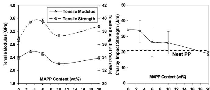
Fig.2 Mechanical properties of 5 wt% filled PP/clay nanocomposites.
