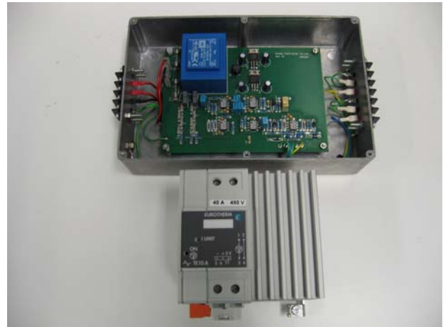
Figure 10: Voltage Control System and Commercial 480Vac, 40Arms Thyristor Phase Controller.
