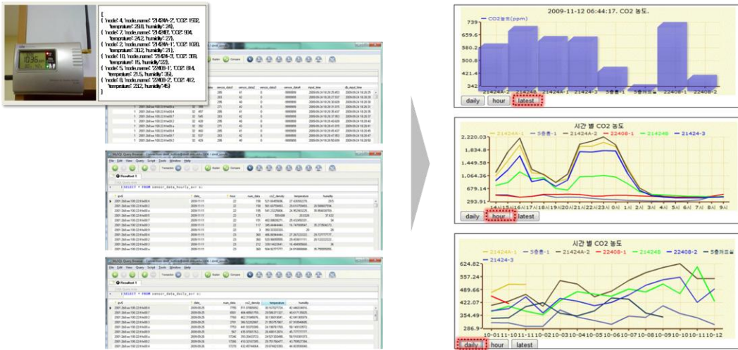
Figure 7 Raw sensing data is visualized in diverse ways: a Bar graph and line graph, daily, hour, and latest time selections.
