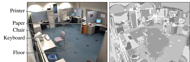
Figure 3. Example region segmentation (important objects are circled). Note that segmentation is quite rough, with the printer and chair broken up into several regions.
