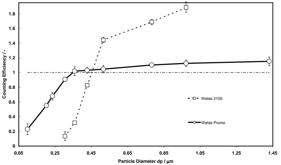
**Figure 2:** Comparison of the counting efficiency of the WELAS 2100 (analogue) (dashed line) and the WELAS 2100 Digital (solid line). (measured using PSL)
