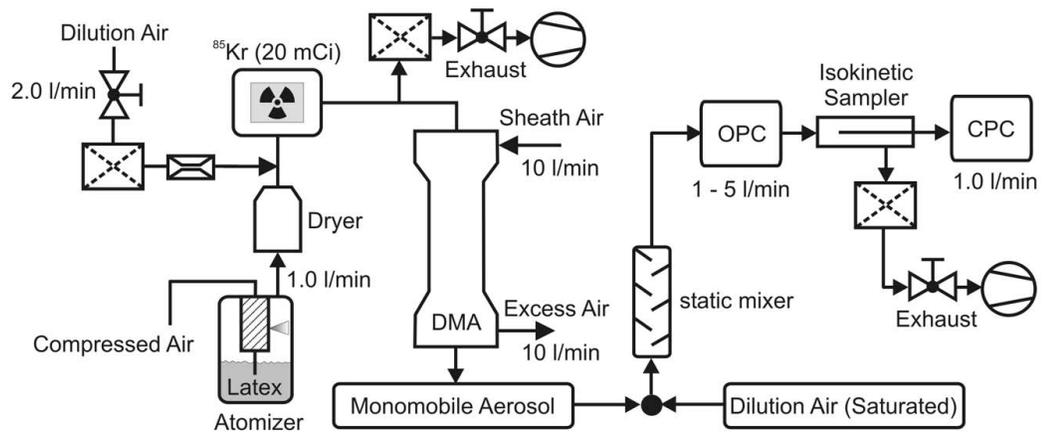
**Figure 1:** Experimental apparatus used for calibration experiments
