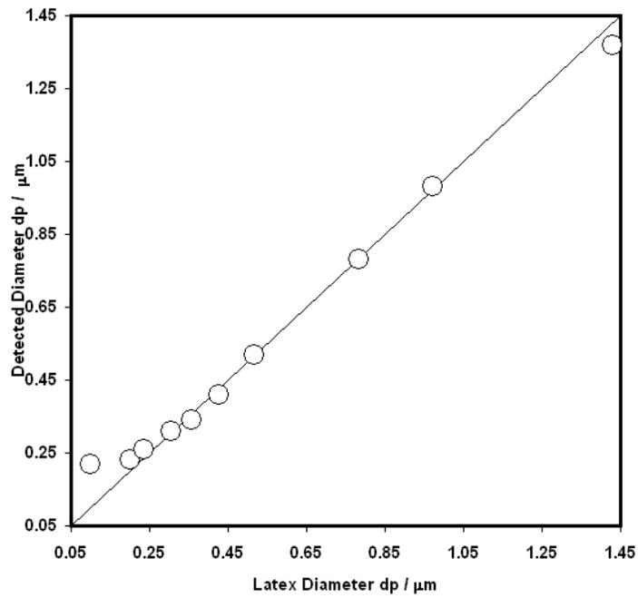
**Figure 3:** Sizing Accuracy of the WELAS 2100 Digital for PSL.
