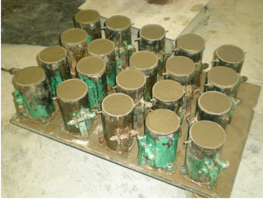
Figure 1. Concrete cylinder specimens after casting
