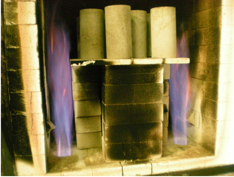
Figure 3. Cylinder specimens set up in furnace for fire exposure
