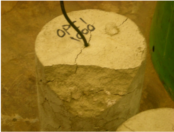
Figure 11. Cracking and spalling of OPC concrete after 1000 °C exposure
