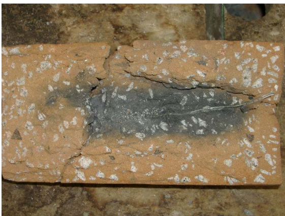
Figure 12. Longitudinal section of geopolymer concrete after 1000 °C exposure
