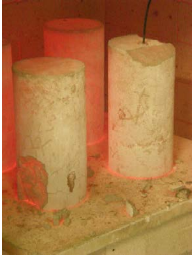
Figure 10. Cracking and spalling of OPC concrete after 800 °C exposure
