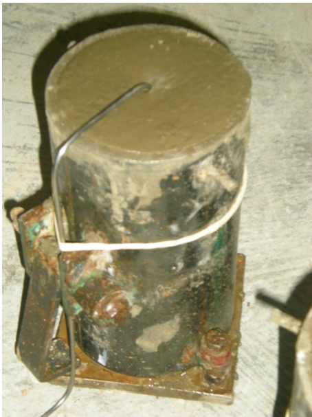
Figure 2. A typical concrete cylinder with thermocouple
