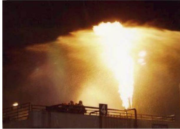
Figure 8 Flange Fire Simulator
