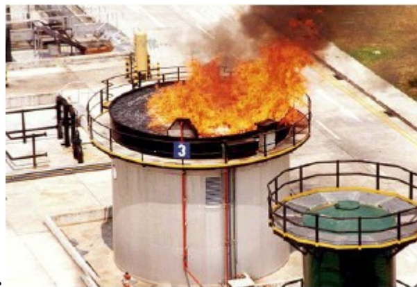
Figure 5 Oil Tank Simulator
