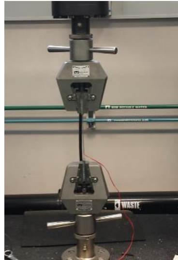
b) Detail of clamp and specimen
