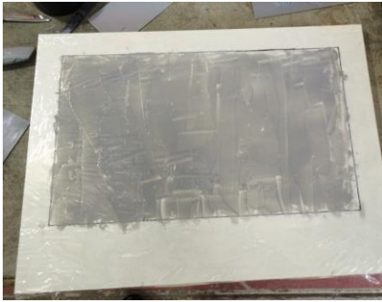
a) Spread epoxy on base board
