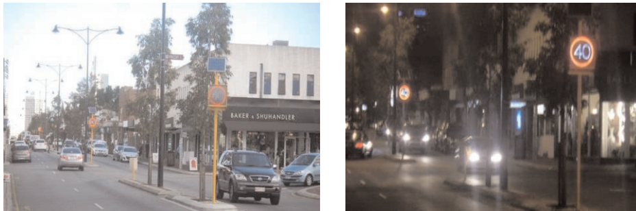
Figure 2. Electronic 40 km/h signs at the same location at day and at night
