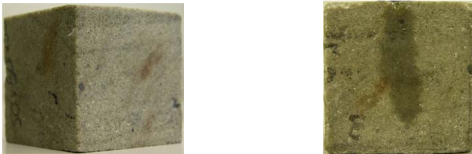
Figure 5: A 5 cm tight sandstone cube before (left) and after (right) hydraulic fracturing experiment.
