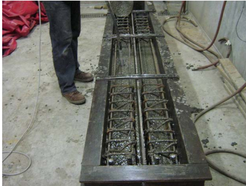
Figure 3.10: Casting and Compacting Geopolymer Concrete
