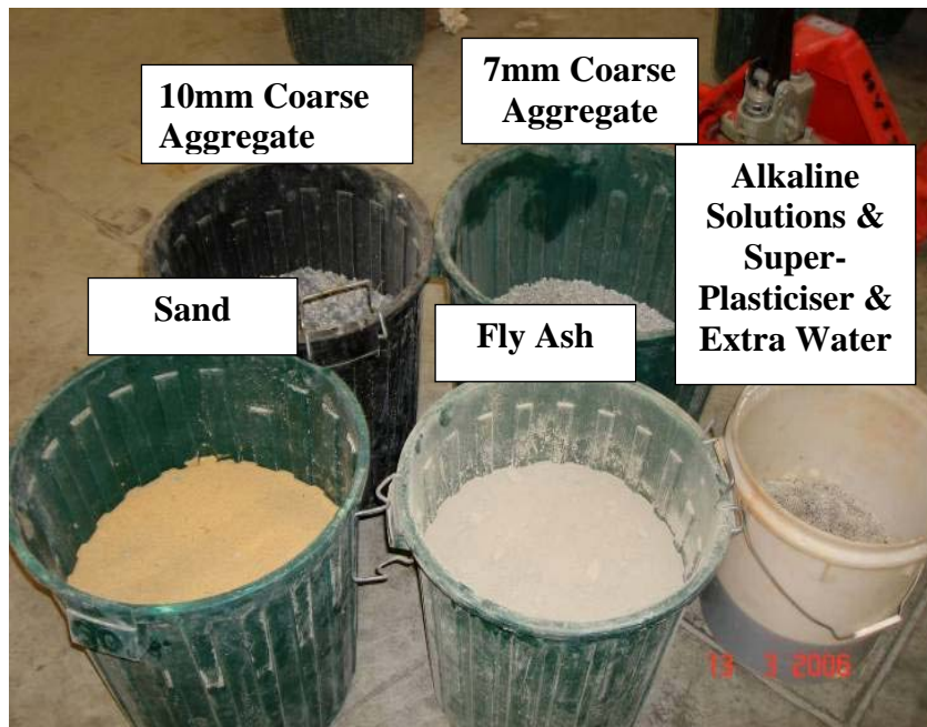
Figure 3.7: Materials for making Fly Ash- Based Geopolymer Concrete
