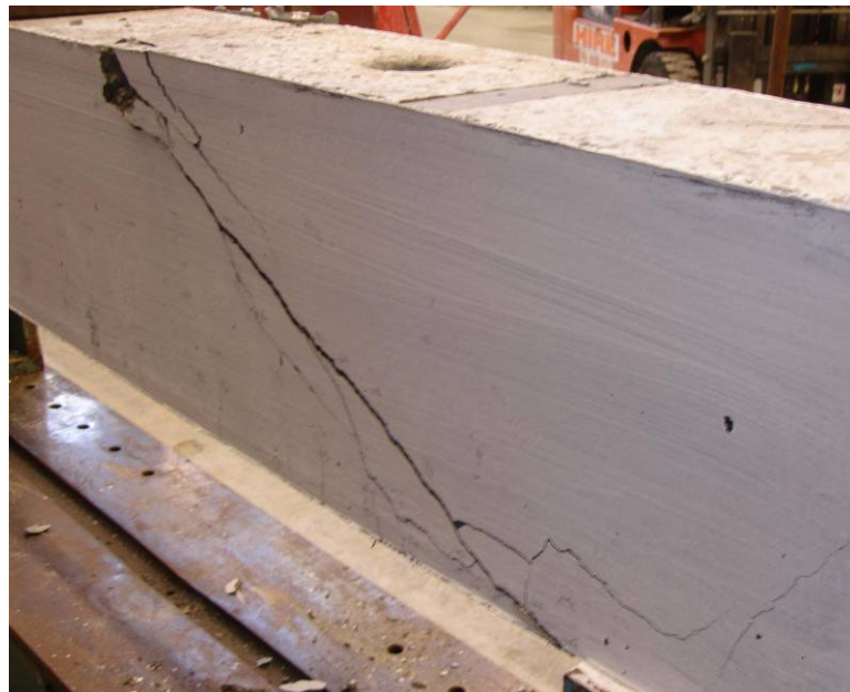
Figure 4.22: Principal Diagonal Crack for Beam S3-2
