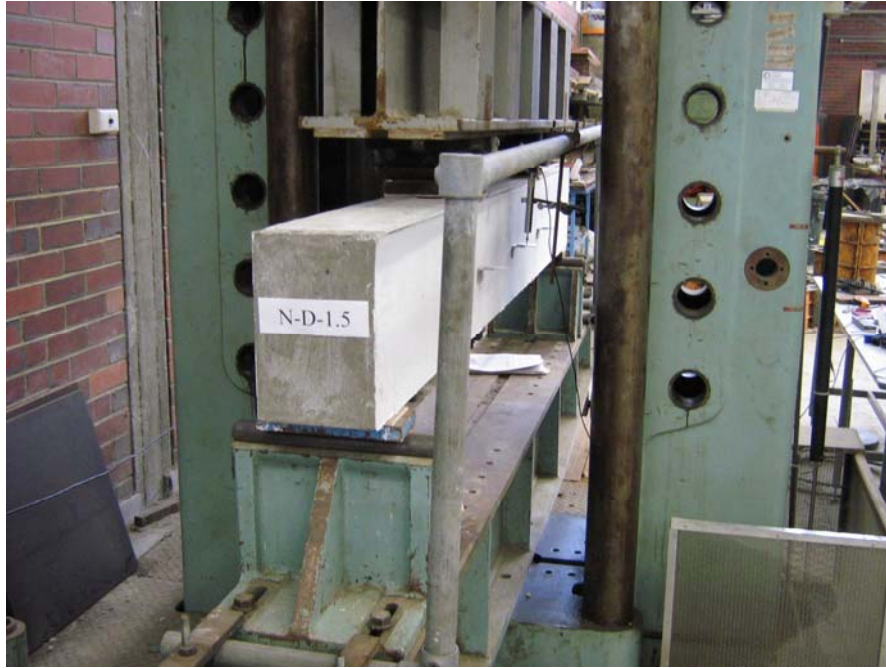
Figure 7.10: Typical Test Set-Up for Beam Tests
