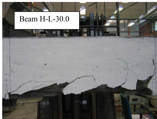
Figure 8.6 : Crack Pattern of High Strength Geopolymer Concrete Beams over the Splice Region After Failure (L-Series)
