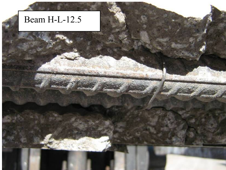
Figure G.4: Steel-Geopolymer Concrete Interface for Beam N-L-12.5 and H-L-12.5
