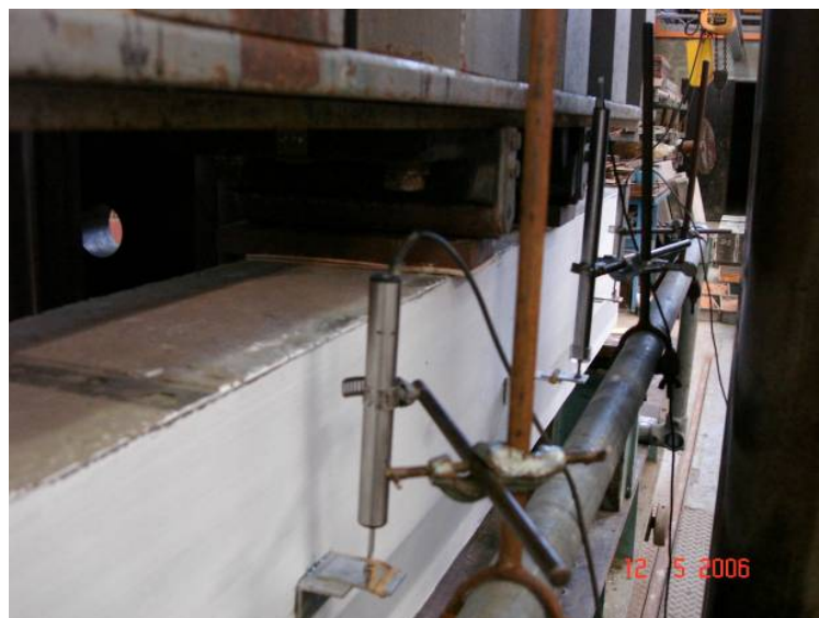
Figure 3.17: LVDTs for Vertical Displacement Measurement
