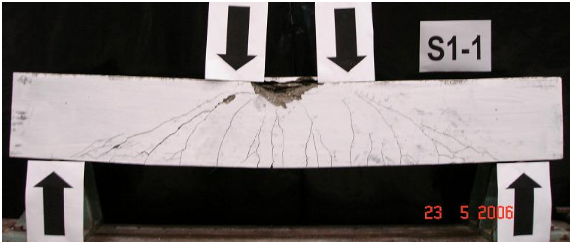
Figure 4.3: Overall Crack Pattern for Beam S1-1 (Back Face)
