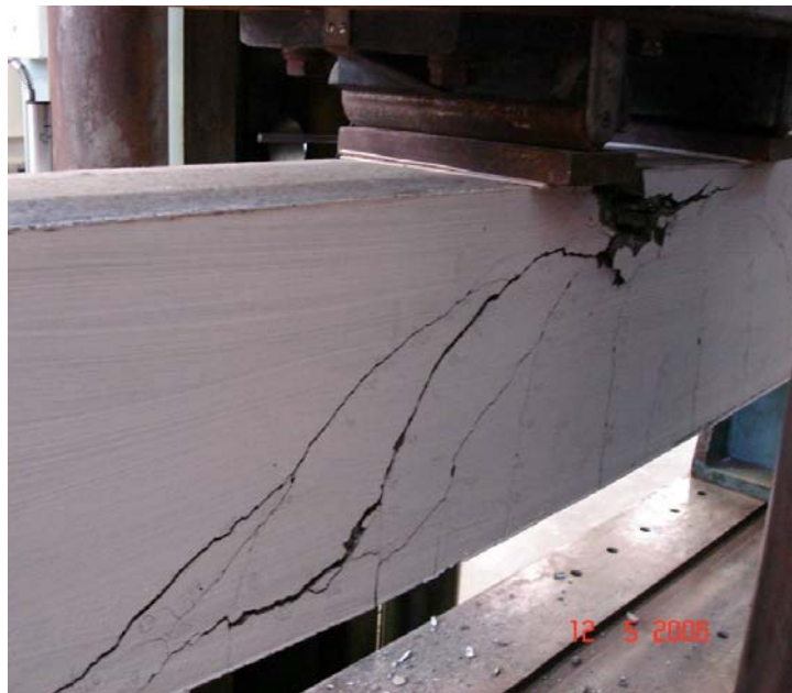
Figure 4.16: Concrete Crushing in Compression Zone for Beam S2-3
