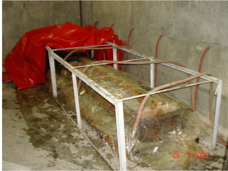
Figure 3.11: Typical Set-up of Steam Curing Chamber
