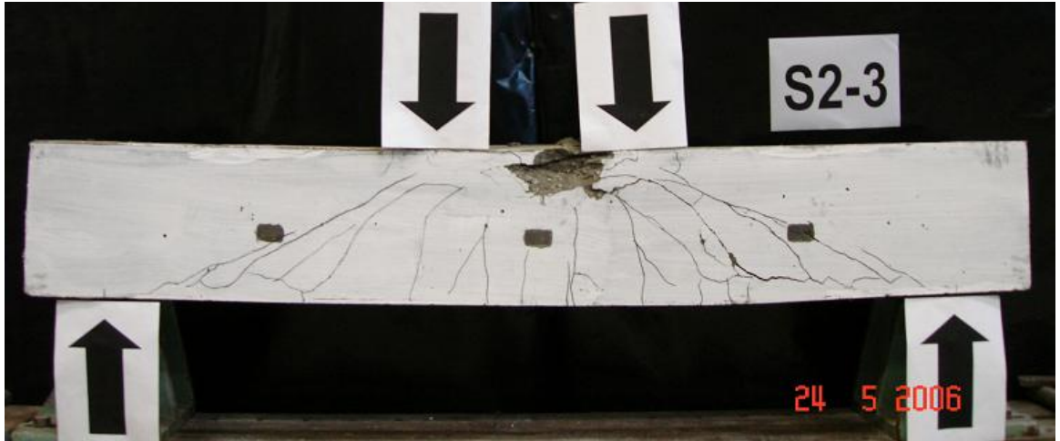
Figure 4.17: Overall Crack Pattern for Beam S2-3 (Front Face)
