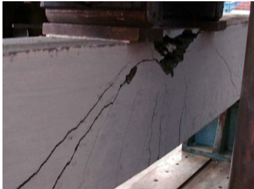
Figure 4.1: Concrete Crushing in Compression Zone for Beam S1-1
