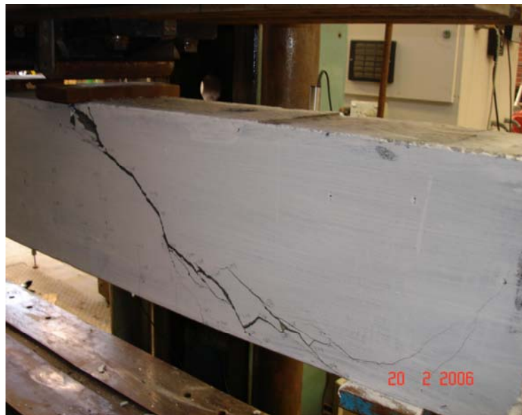
Figure 4.19: Principal Diagonal Crack for Beam S3-1
