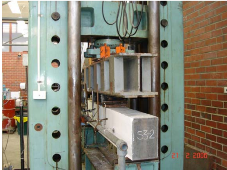
Figure 3.16: Typical Test Set-Up for Beam Tests
