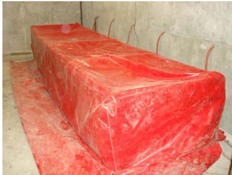
Figure 3.13: Complete Set-Up of Steam Curing Chamber
