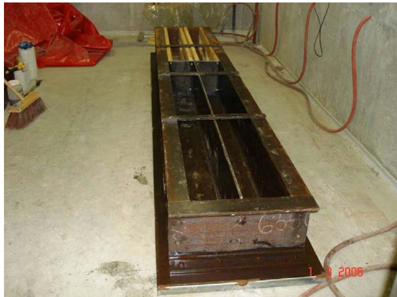
Figure 3.5: Mould for Beam Specimens
