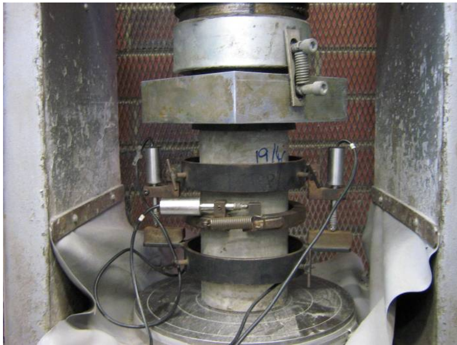
Figure 7.8: Typical Test Set-Up for Modulus of Elasticity of Concrete and Poisson Ratio
