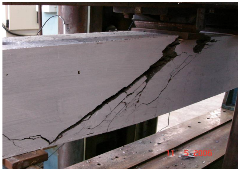
Figure 4.25: Principal Diagonal Crack for Beam S3-3
