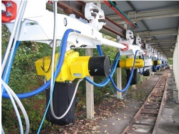
Figure 2.8: Monorail system hoist unit
