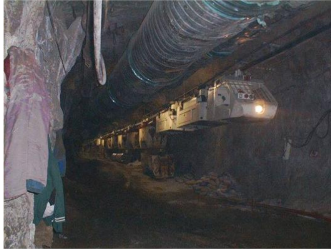
Figure 2.2: EMTS in an underground haulage (Courtesy – Scharf, 2007).
