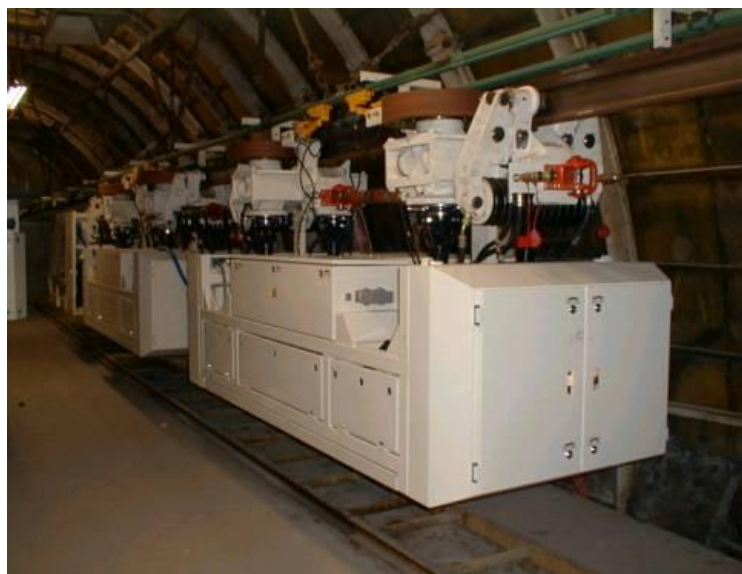
Figure 2.6: Power pack for monorail train (Courtesy – Scharf, 2007)
