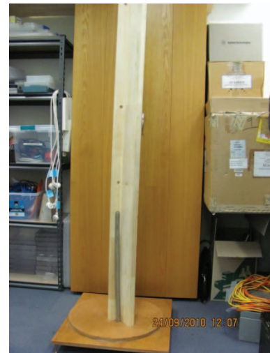
Fig. 2. Photograph of wooden mast, for the antenna under test, with manual rotation
