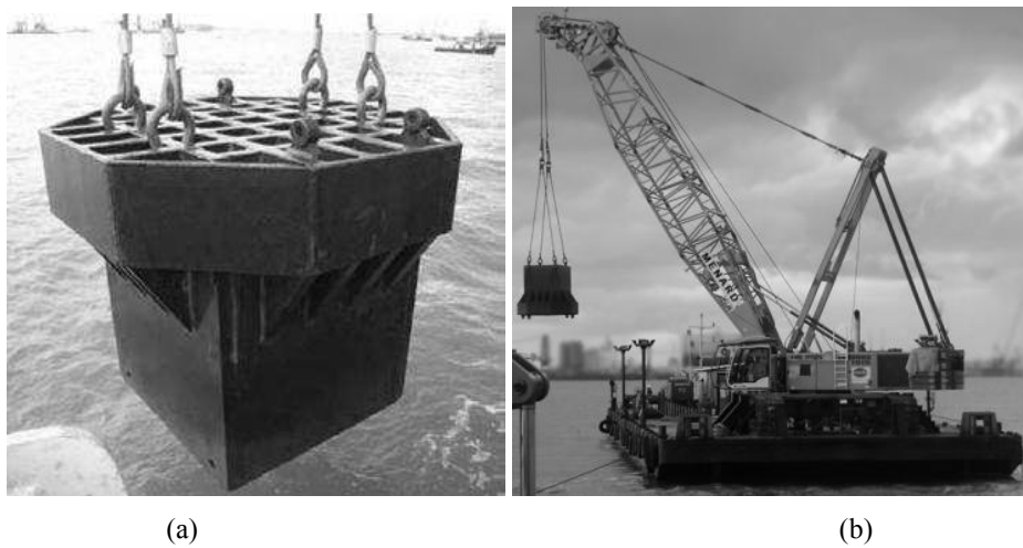
Figure 4: (a) Marine DR (bottom side) - DC (top side) pounder (Chu et al., 2009), (b) barge mounted crane used for offshore dynamic replacement (Hamidi et al., 2010)
