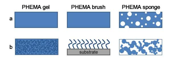
Figure 4.1: The different forms that PHEMA has been synthesised as. a) macroscale schematic of the different forms of PHEMA, gel and brush surfaces are smooth and continuous, sponge PHEMA has large pores, b) microscale schematic showing the difference in the arrangement of the polymer.
