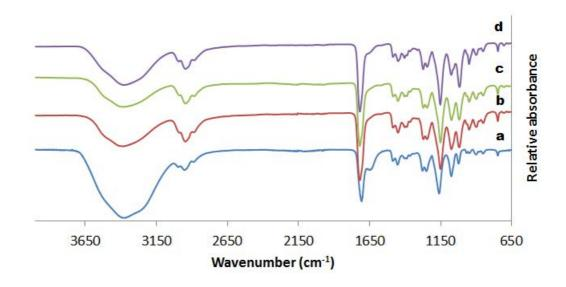
Figure 2.6: ATR-FTIR spectra of PHEMA (a), P(HEMA:GMA) (b), P(HEMA:GMA)-NH<sub>2</sub> (c) and P(HEMA:GMA)-HS (d).
