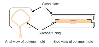
Figure 2.1: Diagram of the hydrogel mould.
