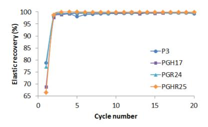
Figure 2.12: Elastic recovery of hydrogels after repeated application of stress at 37°C. Stress of 10 Pa was applied over 30 s followed by a recovery of 240 s.
