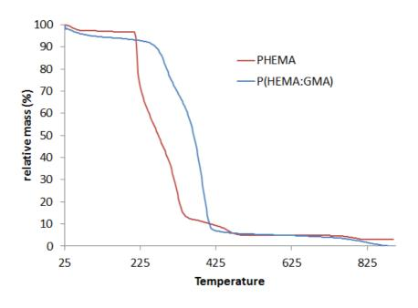
Figure 2.8: TGA curves for PHEMA and P(HEMA:GMA).
