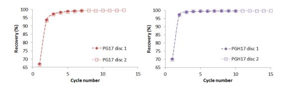
Figure 2.11: Elastic recovery of hydrogels after application of repeated stress at 20℃. Stress of 10 Pa was applied over 60 s (30 s for P(HEMA:G MA)) followed by a recovery of 240 s.
