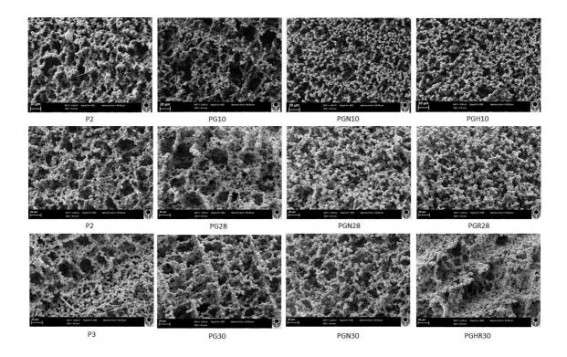
Figure 2.10: SEM images of the cross-sectional area of hydrogels. All images were taken at 3keV with a working distance of 5.0 mm giving 500x magnification, the scale bar was 20  $\mu\text{m}.$
