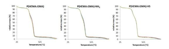
Figure 2.9: TGA curves for 3 batches of hydrogel showing low batch-to-batch variability. PG10 (red), PG12 (blue) and PG23 (green).
