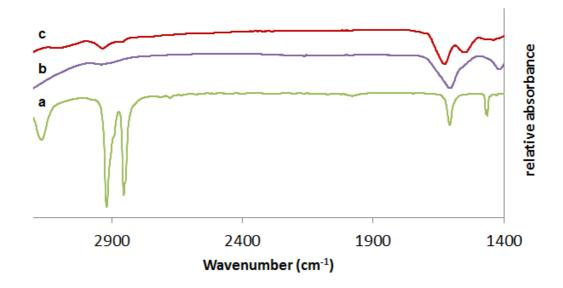
Figure 2.7: ATR-FTIR spectra demonstrated the reaction of HS with hexamethylenediamine. Hexamethylenediamine (a), HS (b) and aminated HS (c).
