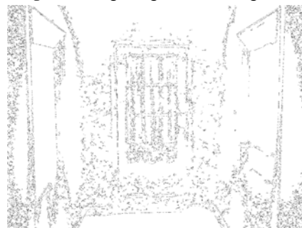
15 Figure 6b Edge diagram of the processed image
