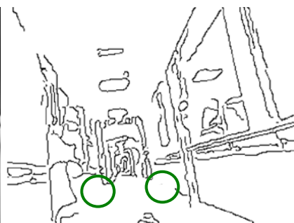
Figure 1b Edge diagram of the original video frame; Canny edge detector (Canny, 1986) was used.
