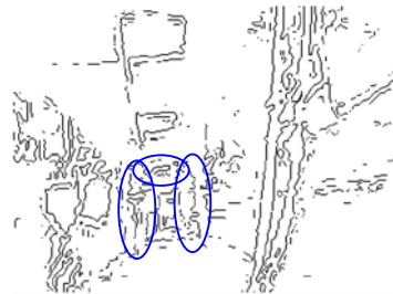
Figure 22c Entry detection: Sobel algorithm after Whyte et al.'s filter.
