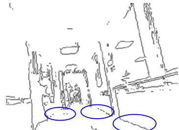
Figure 17d Corridor detection: Sobel algorithm within the proposed MFS framework.
