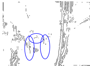
Figure 22b Entry detection: Sobel algorithm after deconvolution filter.
