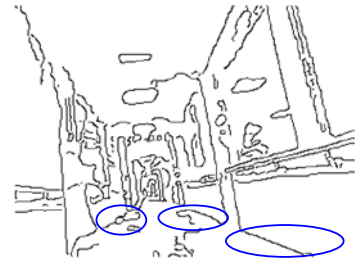
Figure 16d Corridor detection: Canny algorithm within the proposed MFS framework.
