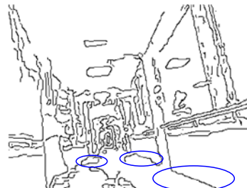
Figure 16c Corridor detection: Canny algorithm after Whyte et al. filter.
