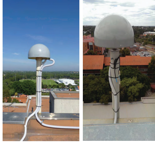
Fig. 1 CUCC (Left) and CUBB (Right) stations at Curtin University equipped with JAVAD TRE_G3TH_8 receivers, connected to TRM59800.00 SCIS antennas.
