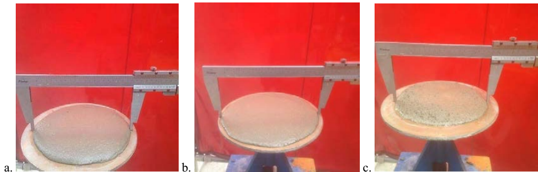
Fig. 2. Flow test (a) 100% sand; (b) 50% FNS and 50% sand (c) 100% FNS
