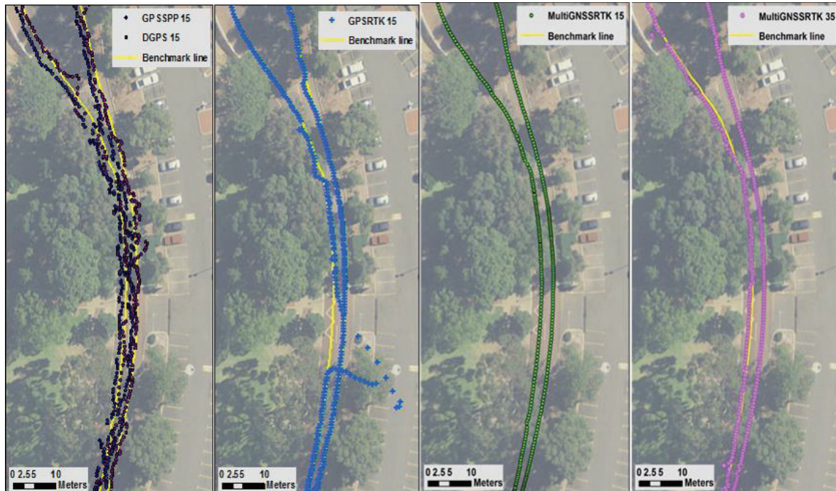
Fig. 4 Comparison of tracking quality of GPS/multi-GNSS with different positioning solutions in a harsh environment with tree canopies
