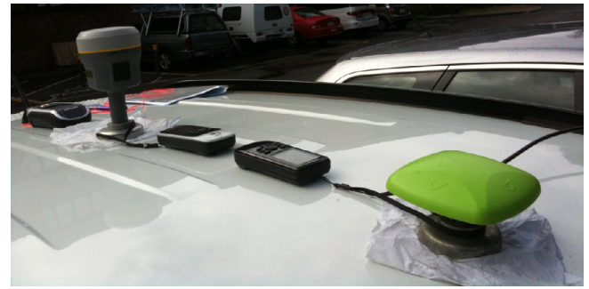
Fig. 3. Experimented GPS receivers and the placement for recording vehicle movement (left to right: Mobilemapper 100, Trimble R10, Garmin76, Garmin 72H, and JAVAD DELTA-3. Receivers were aligned in the middle of the car roof; the distances between receivers were measured).
