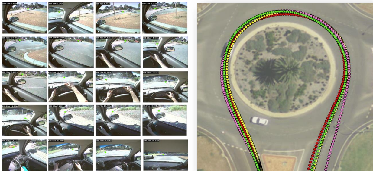
Figure 2. Sample eye fixation video frames at a U-turn manoeuvre from one participant (left) and vehicle movement trajectories from five participants (right), adapted from (Qian Sun, Jianhong (Cecilia) Xia, Nandakumaran Nadarajah, et al., 2016)
