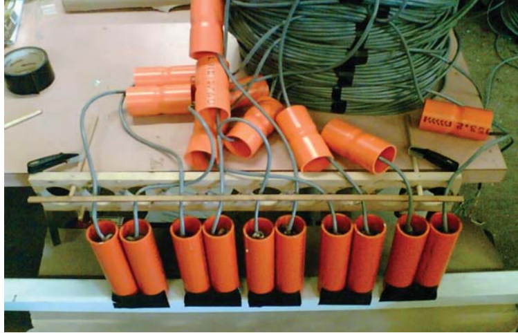
Figure A4.16. Epoxy resin encapsulation “potting” of geophone sondes in 50mm electrical conduit for installation into boreholes.
