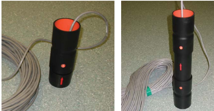
Figure A4.17. PCB 500g tri-axial accelerometer sonde (left) and OYO101LT 14Hz tri-axial geophone sonde (right) in 63mm conduit for installation into boreholes.
