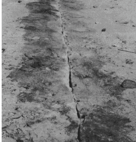
Figure 3.6. Fracture created by pre-splitting in Lithonia granite (Devine et al., 1965)
