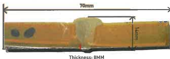
Figure 15: Typical sample of welded, rich grade, 13Cr martensitic stainless steel.
